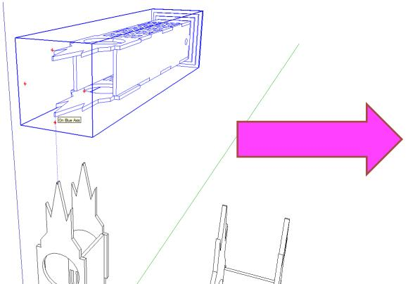
Click on the move tool and move the lamp so the corners of the base meet and then separate again
