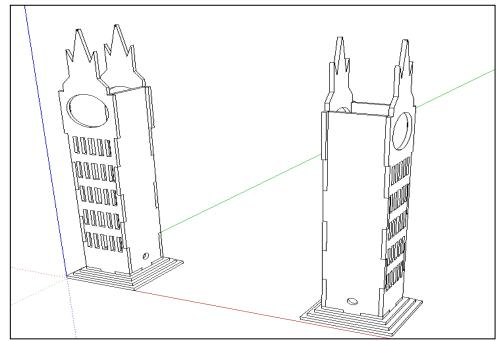
Click on the move tool and move the lamp so the corners of the base meet
