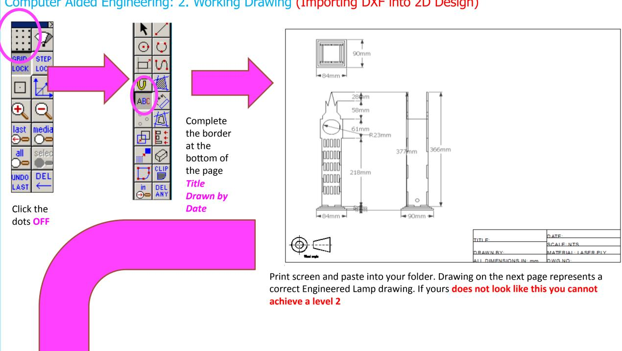
Computer Aided Engineering: 2. Working Drawing (Importing DXF into 2D Design)
