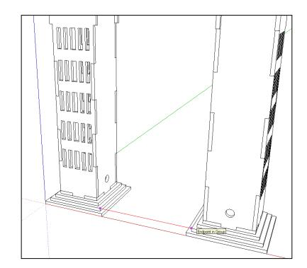
Click on the move tool along the red axis. You should be able to draw a line that turns red from corner to corner to indicate it lines up exactly
